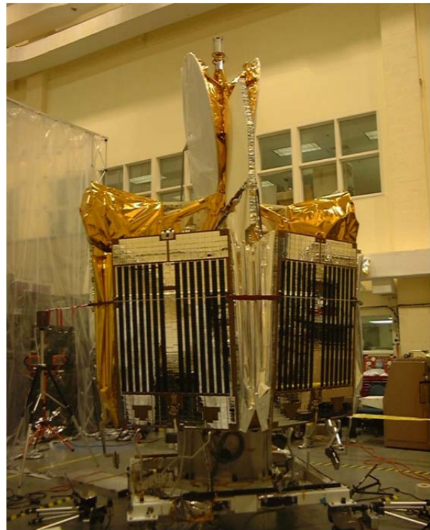
Figure 51: Picture of the WMAP spacecraft with its deployable solar array/sunshield stowed. This design is the heritage for the DRM2 solar array/sunshield concept.
